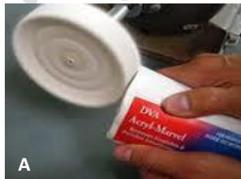
A- Muslin buffing wheel attached to dental lathe. B- Rouge
